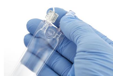
Figure 6: OFM Perfusate Bag without air bubbles.
