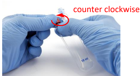
Figure 2: Remove red protection cap from the OFM Perfusate Bag.
