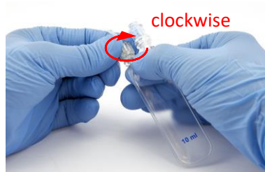
Figure 3: Connect the OFM Perfusate Bag via luer-connector with the PUSH-part of the OFM Tubing.
